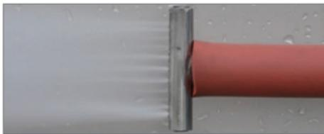
※ Flat nozzles are suitable for HVAC cleaning
