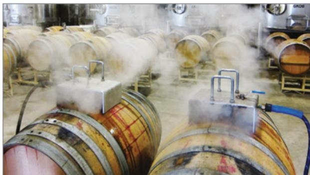
※ Using the OPTIMA STEAMER and our Barrel Cleaning Tool will use a fraction of the water you would use with a pressure washer, while killing more bacteria in the surface of the barrel and penetrate deeper. Produce swell in minutes - not hours - while preserving toasting flavors and character rather than flushing them away.
